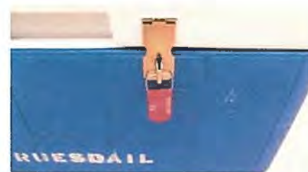
Outside of cooler with plastic security tag affixed
